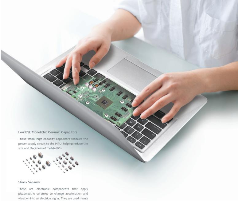
with HDDs as sensors for preventing the writing of data when an impact is received from an external source.
