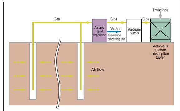
\*\* Water pumping, aeration and activated carbon absorption process
