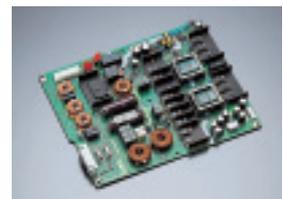
Switching Power Supply for Flat Panel Display
