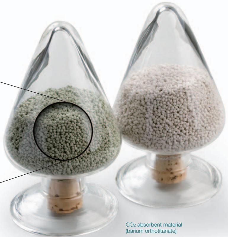
CO<sub>2</sub> absorbent material (barium orthotitanate)
