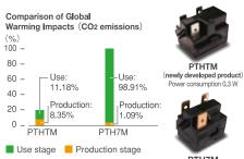
"Calculations are based on the assumption of using the thermistor to start up the motor in a refrigerator over a period of 10 years.
