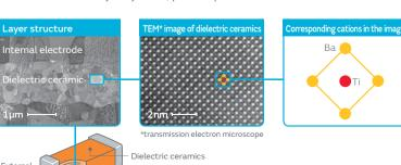
Micro and nano structures in a MI CC (monolithic ceramic capacitor
