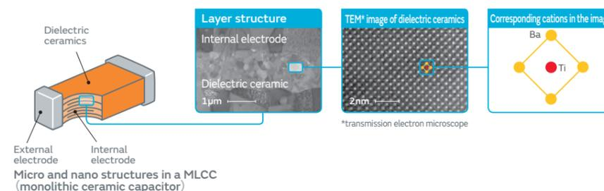
Micro and nano structures in a MLCC (monolithic ceramic capacitor)
