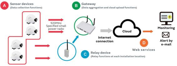
has become increasingly intense, resulting in onset of heat stroke, excess fatigue, and ill health. Accordingly, Murata Manufacturing Co., Ltd., with expertise in offering sensor technology and system solutions, collaborated with TODA CORPORATION to develop a system for monitoring biological information and working environments in August 2018. Looking ahead, we will continue using technologies to address such social issues.
