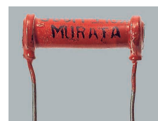
Barium titanate ceramic capacitor
