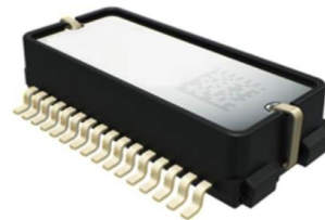
6-DOF XYZ-Axis MEMS inertial sensors
