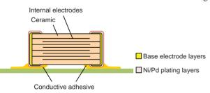
Figure 1: Example structure of the GCB Series
