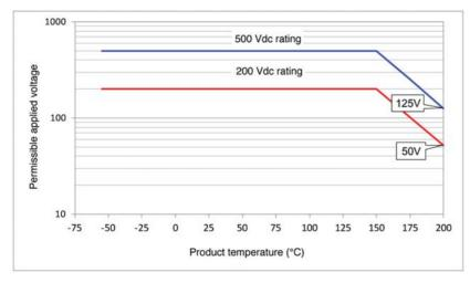
Fig. 3: Reduction of voltages to be applied
