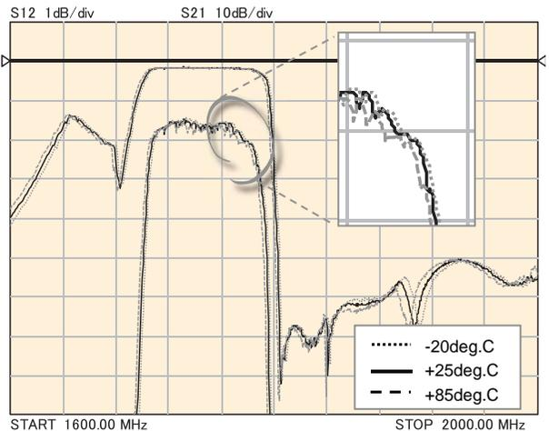
Figure 3: BAND3 transmission properties of SAHRT1G-74BB0B0A
