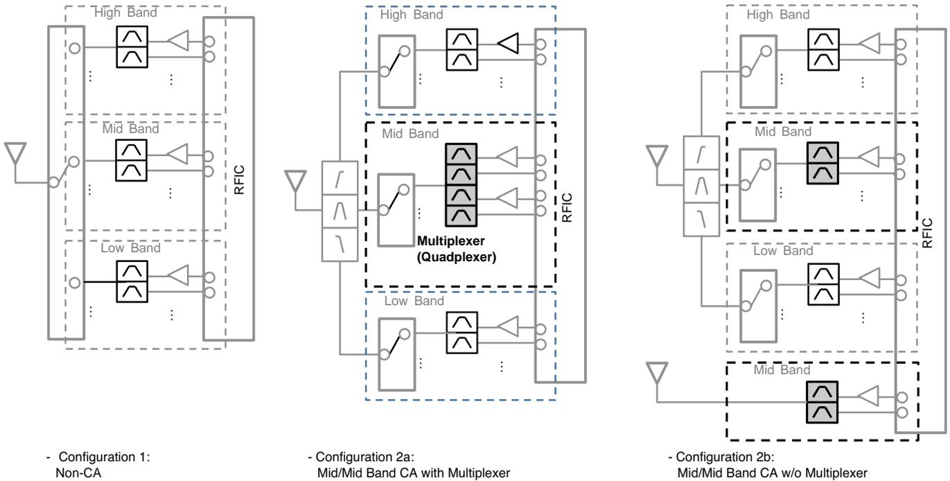
Figure 2: Configuration examples of RF front ends with or without Carrier Aggregation
