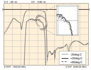
Figure 3: BAND3 transmission properties of SAHRT1G-74BB0B0A
