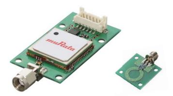
Photo 2: External appearance of the RFID reader/writer module (left) and the small tag reader antenna (right)
