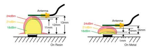
Fig. 3: Schematic for communication distance of LXMS21NCNH-147
