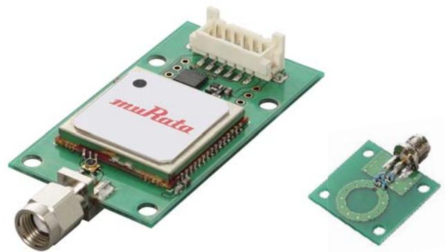
**Photo 2:** External appearance of the RFID reader/writer module (left) and the small tag reader antenna (right)
