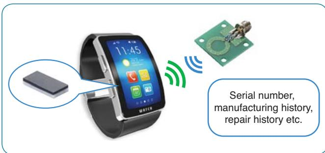
Fig.1: An RFID tag embedded in a small device is being read.
