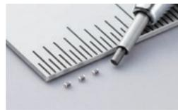
Development of the world's smallest\* UWB modules with acceleration sensors and Bluetooth® Low Energy
